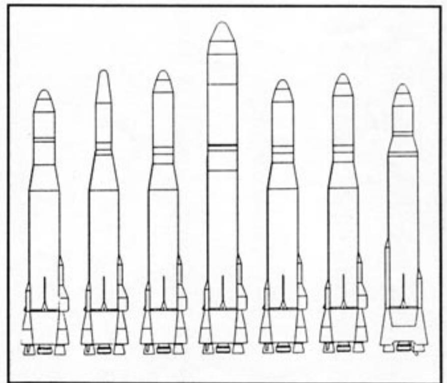
Fig. 12 "The Atlas E/F Pedigree" - Atlas E/F variants from left-to-right (length in parenthesis): OVI and Whitecloud (27.3 m); Burner II (28.9 m); PTS and SVS (29.2 m); Seasat (34.6 m); Tiros-N and DMSP (28.1 m); ATN and Geosat (28.65m); Atlas H (27.4 m).
