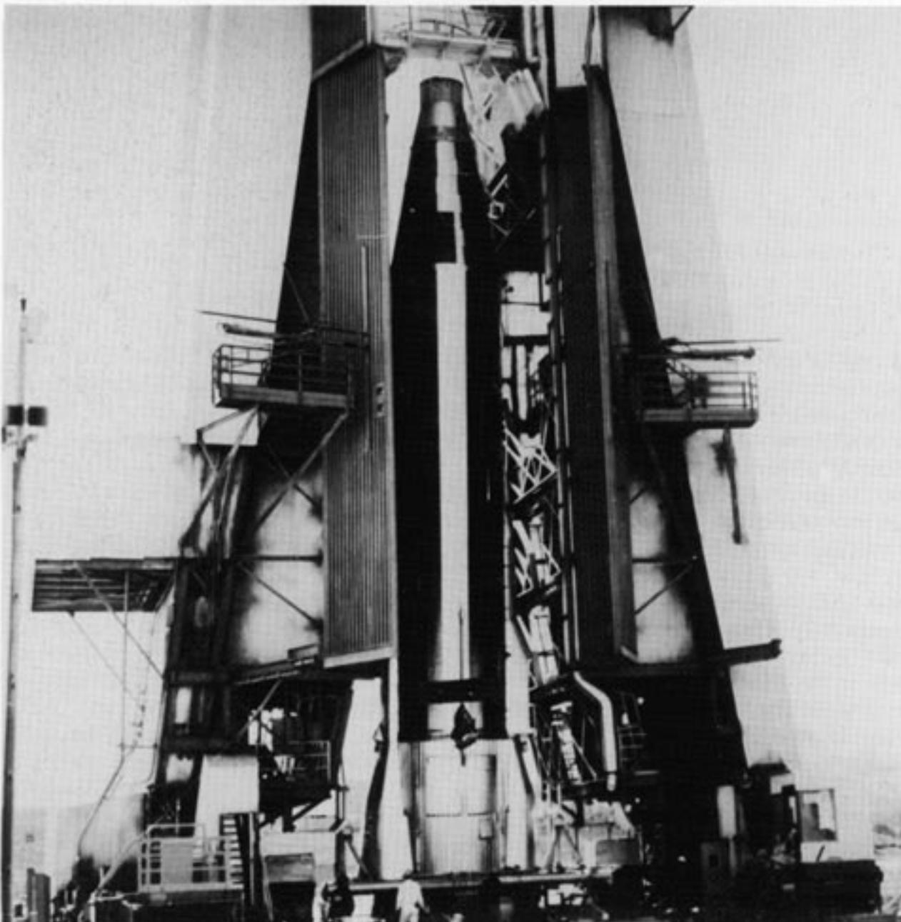
Fig. 8 The Atlas E/F rocket for the NOAA-6 weather satellite is enclosed by the service structure at SLC-3W prior to installation of the payload. (Note the curious and clumsy attempt to cover up what must be the serial number on the centre body of the rocket.) (NASA)
