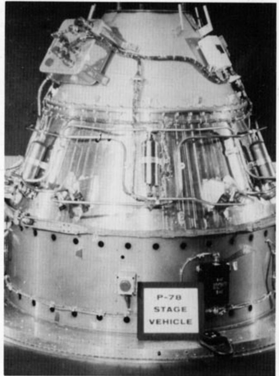
Fig. 3 The Orbit Insertion System (OIS) upper stage. (Fairchild Space Company, courtesy Ed Hengeveld)
