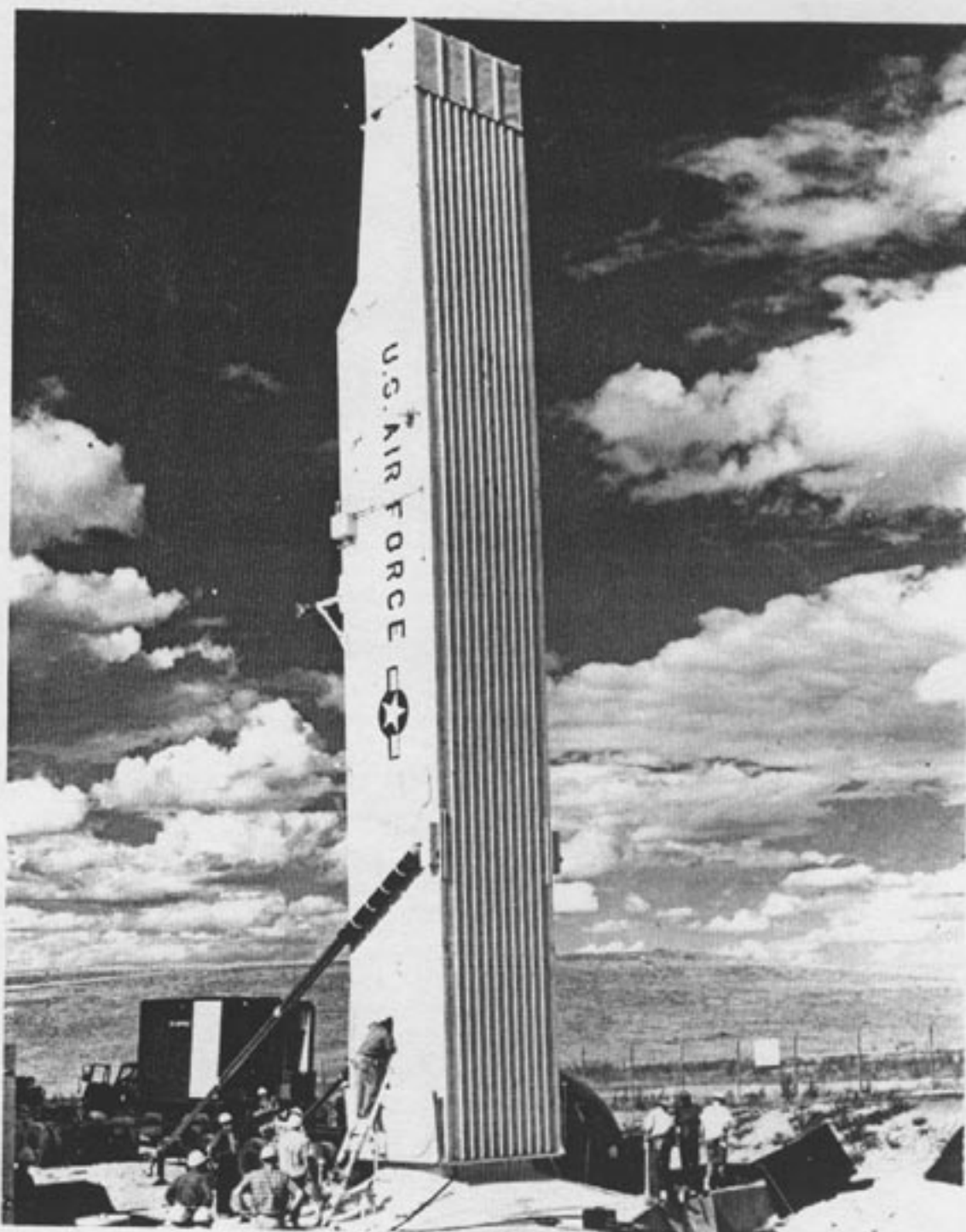
Transporter-erector demonstration near Malmstrom AFB, MT. The huge tractor-trailer, largest vehicle ever designed for regular highway use, was developed by the Boeing Company to transport the missiles to and from underground launchers and place them in the silos.
